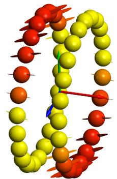
The inner geometry of the rolling bearing is provided by the user, but it can also be approximated from the load capacities by the software. The calculation returns the pressure distribution between the rolling elements and the reference life according ISO/TS 16281 for a given loading (force and moment or tilting).
